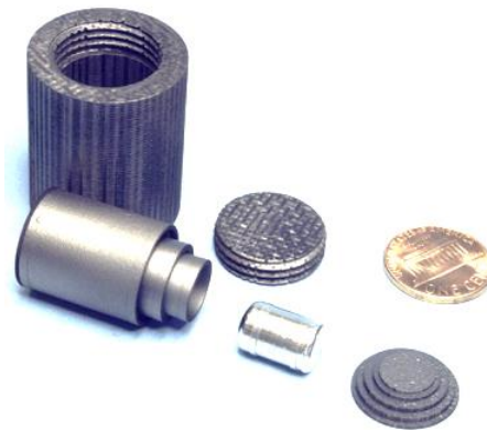
Figure 3-2. LWRHU- light-weight radioisotope heater unit, components
